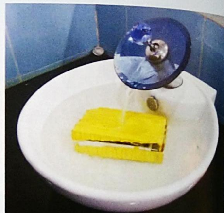
裸露的電池被水完全浸泡 Uncovered cell gets fully soaked by water
