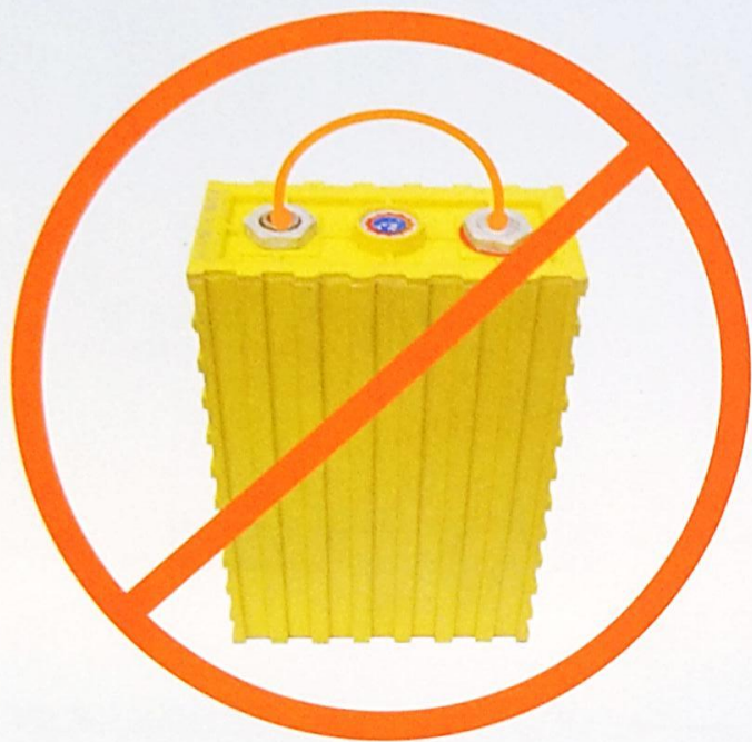
電池短路 Battery short circuit
